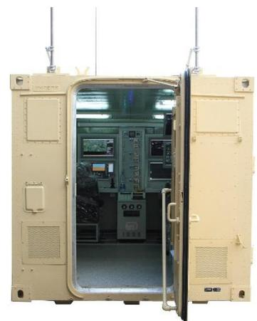
**Ground control station** can be easily and effectively integrated into the existing network systems, disseminating necessary information between users-eg. transmission of the intelligence information from the GCS to the headquarters while operations preparation
